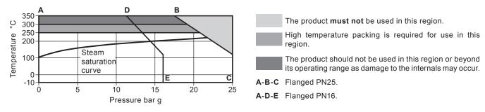
Note: As standard the XYZ series two port control valves are supplied with PTFE stem seal and metal-to-metal seats.
