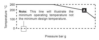
A Is the maximum allowable temperature (TMA) the body of the product can be raised to permanently, at a given pressure.
