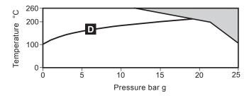
**D** The steam saturation curve is added (where relevant) to enable users to easily find the specific operating points, e.g. 10 bar g saturated steam @ 185 °C, 10 bar g steam with 20 °C superheat or 10 bar g / 250 °C steam.
