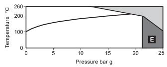
E Sometimes end connections or internal components may restrict the operating envelope of the product below the standard rating. Care must therefore be taken in selecting appropriate end connections. In this case the product should not be used in area 'e' and will be worded:
