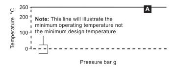
Is the maximum design temperature the body of the product can be raised to permanently, at a given pressure.
