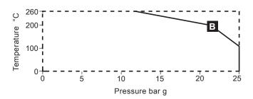
**B** Is the maximum allowable pressure (PMA) which can be tolerated within the body of the product at a given temperature. It is a function of the PN rating and body design / material.
