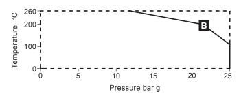
**B** Is the maximum design pressure that the combined body and end connections of the product can withstand at a given temperature. It is a function of the PN rating and body design / material.
