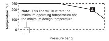
A Is the maximum design temperature the body of the product can be raised to permanently, at a given pressure.
